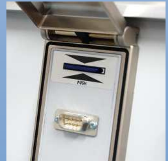
extern Data storage unit
